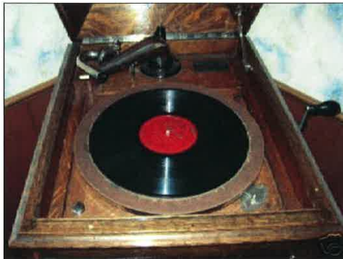
This is how it held the record and you can see the crank on the right that created the power to play the record.
